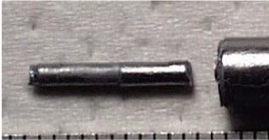
Fig. 6. Photos of seeding part of TLZ grown crystals.
