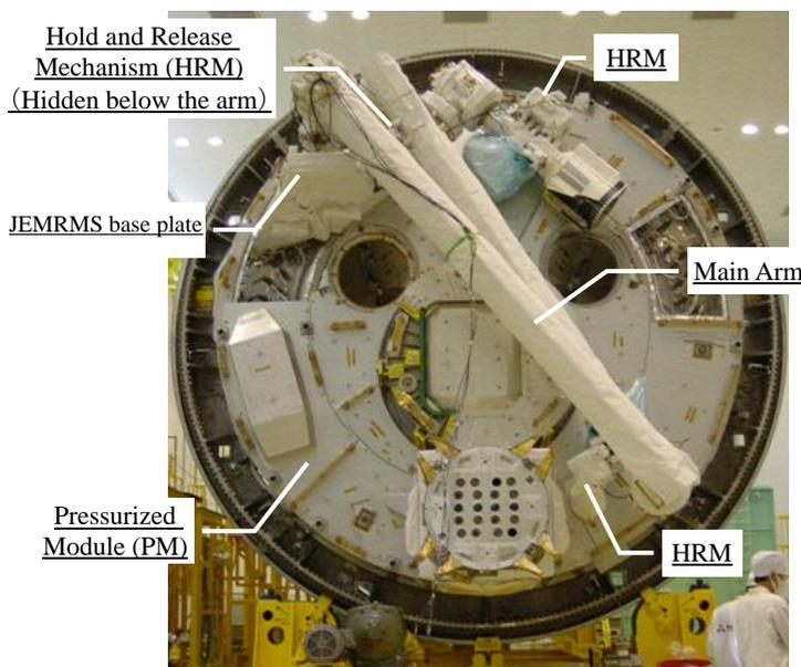
Figure 4.5.3-1 JEMRMS locked to PM (Launch configuration)
