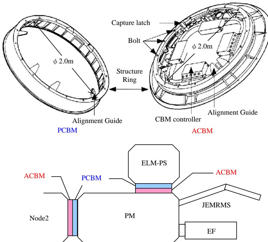
Figure 4.1.3-1 Common Berthing Mechanism (CBM)
