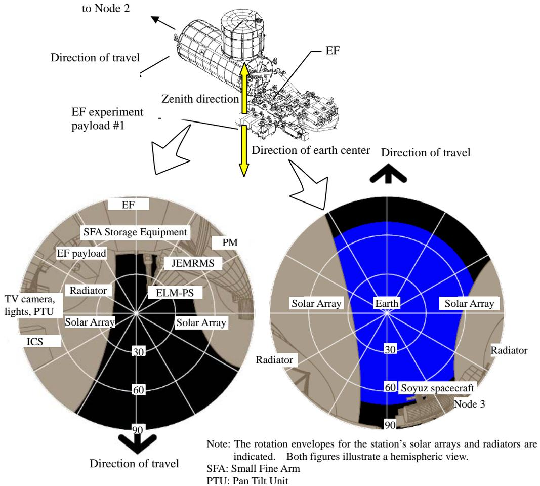
Figure 6.2.2-1 Estimated field of view for EF experiment payload #1 site on EF
