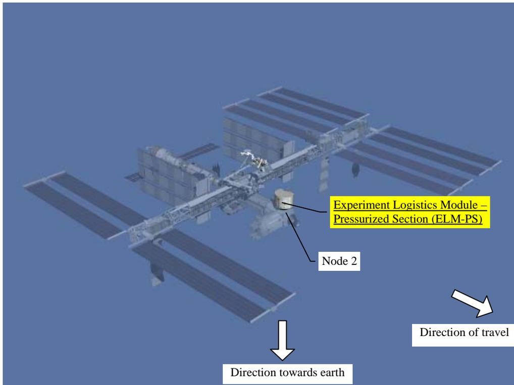
Figure 5.2.1-1 ISS after completion of IJ/A Flight
