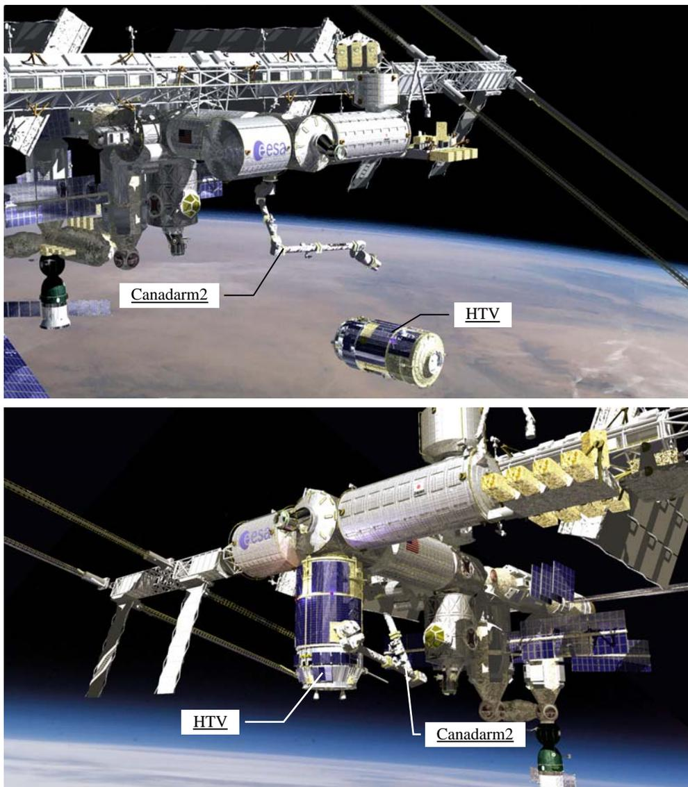
Figure 7.2.3-2 Images of HTV approaching the ISS (above) and HTV Berthing to the ISS (below)
