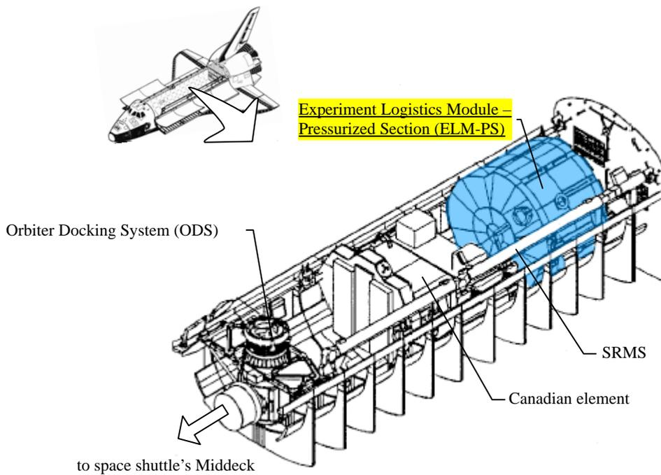
Figure 5.2.1-2 Cargo bay layout during launch of IJ/A Flight (Image)
