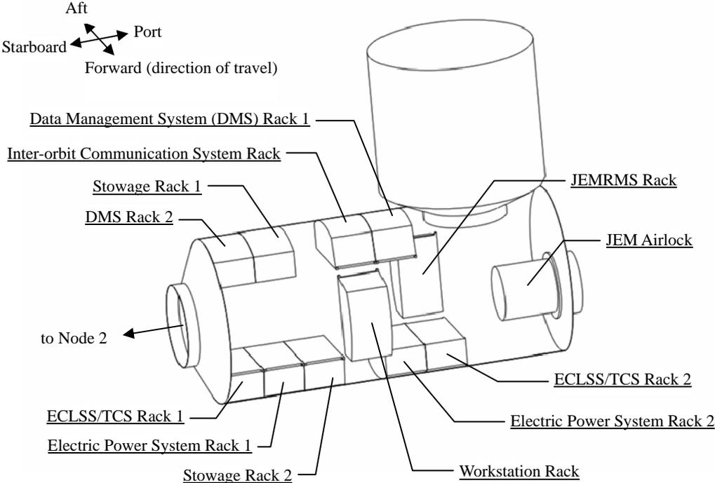
Figure 4.1.2-3 JEM System Racks inside PM
