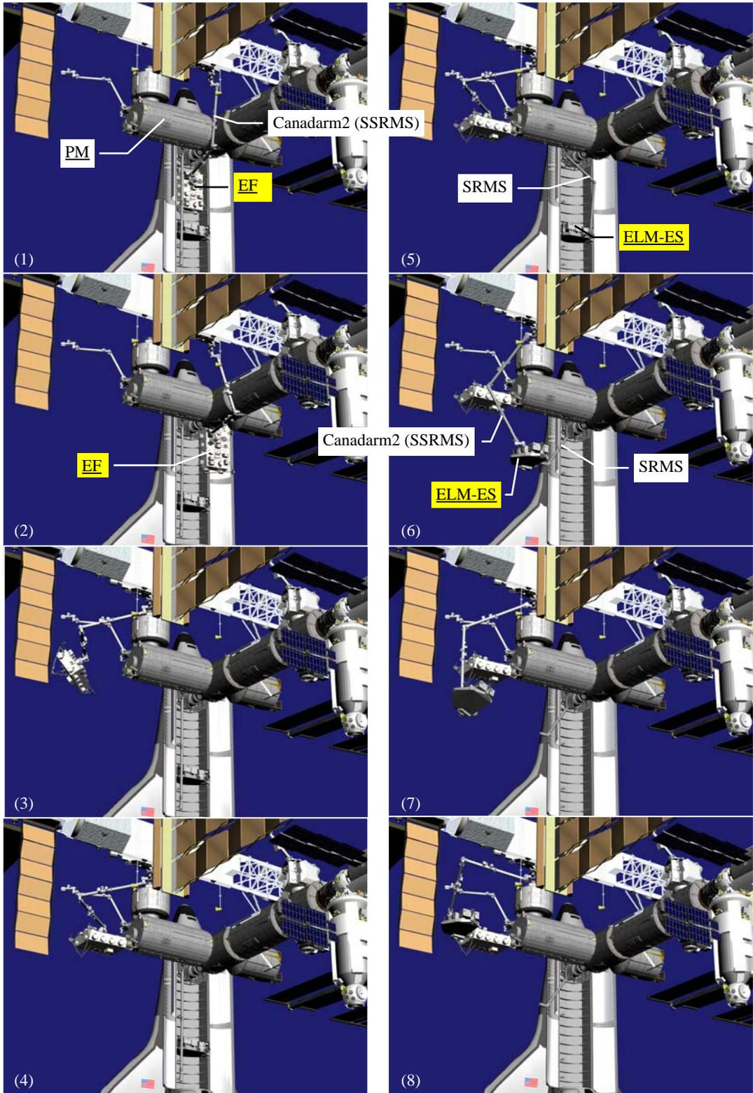
Figure 5.2.3-3 Procedures for connecting EF and ELM-ES to ISS
