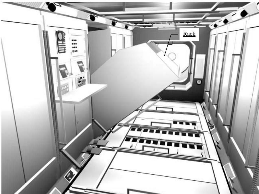
Figure 4.1.2-5 Schematic of how to attach or detach the racks: Each rack can individually be attached and detached for relocation, exchange, or maintenance.
