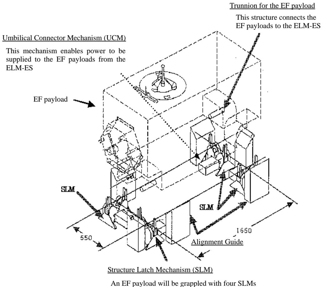
Figure 4.4.3-1 Payload Attachment Mechanism (PAM)
