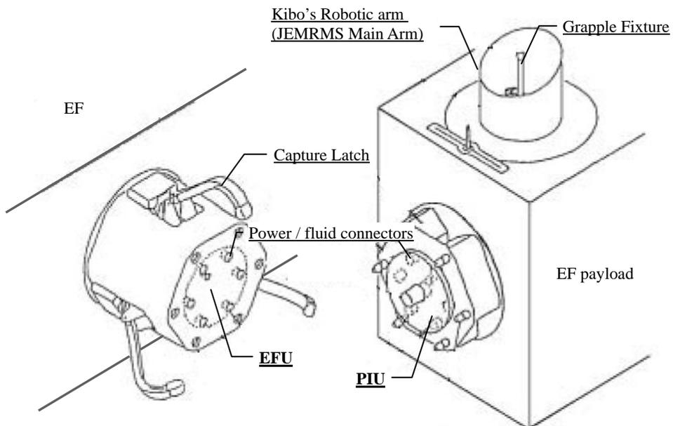
Figure 4.3.3-2 EEU (EFU and PIU) Structures
