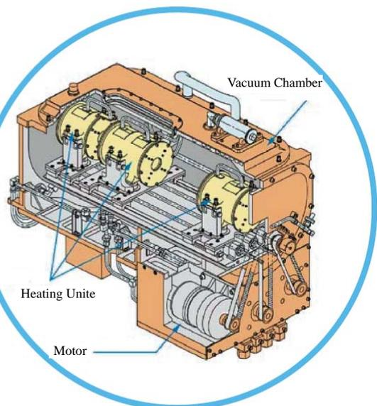
GHF Material Processing Unit (Furnace)
