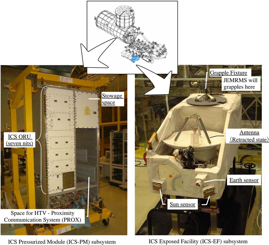
Figure 4.6.2-1 Inter-orbit Communication System (ICS)
