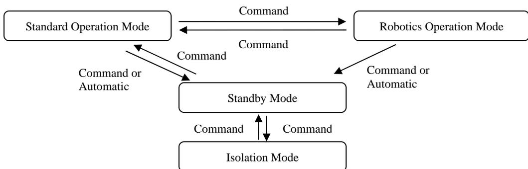
Figure 3.2-1 Kibo Operation Mode Transitions
