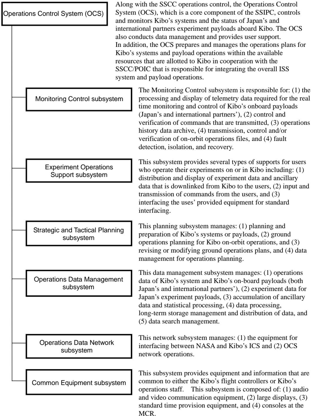
Figure 5.3-2 Kibo Operations Control System
