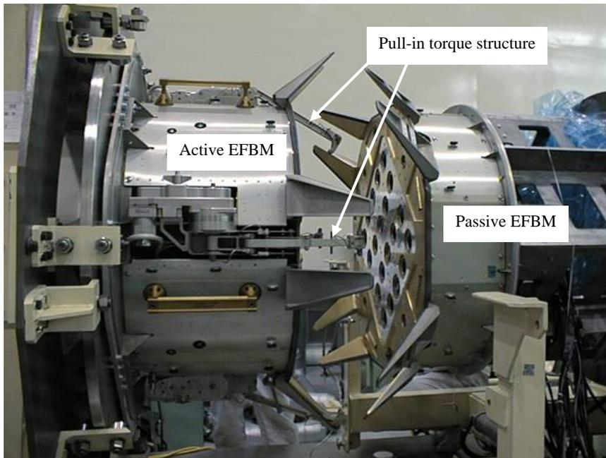
Figure 4.3.3-1 Exposed Facility Berthing Mechanism (EFBM)
