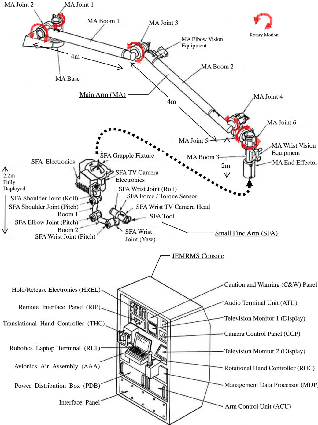
Figure 4.5.2-1 Main Arm (MA), Small Fine Arm (SFA) and JEMRMS Console
