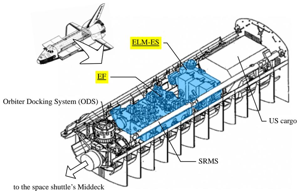
Figure 5.2.3-2 2J/A Cargo bay layout during launch of 2J/A Flight (Image)
