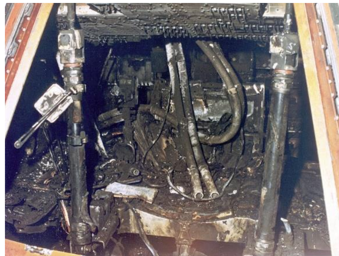
Fire accident on the ground test in "Apollo 1" in 1967.
