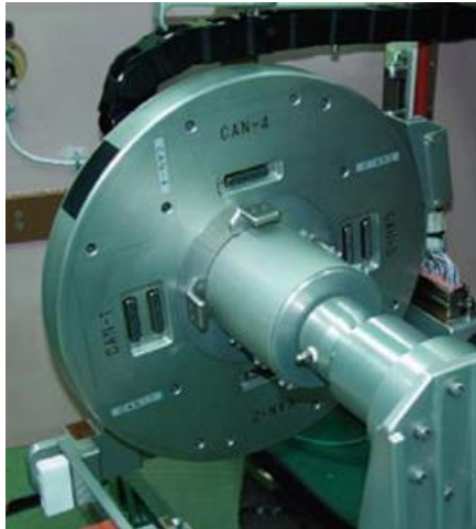
Fig. 2.2-2 Artificial gravity compartment attachment conditions
