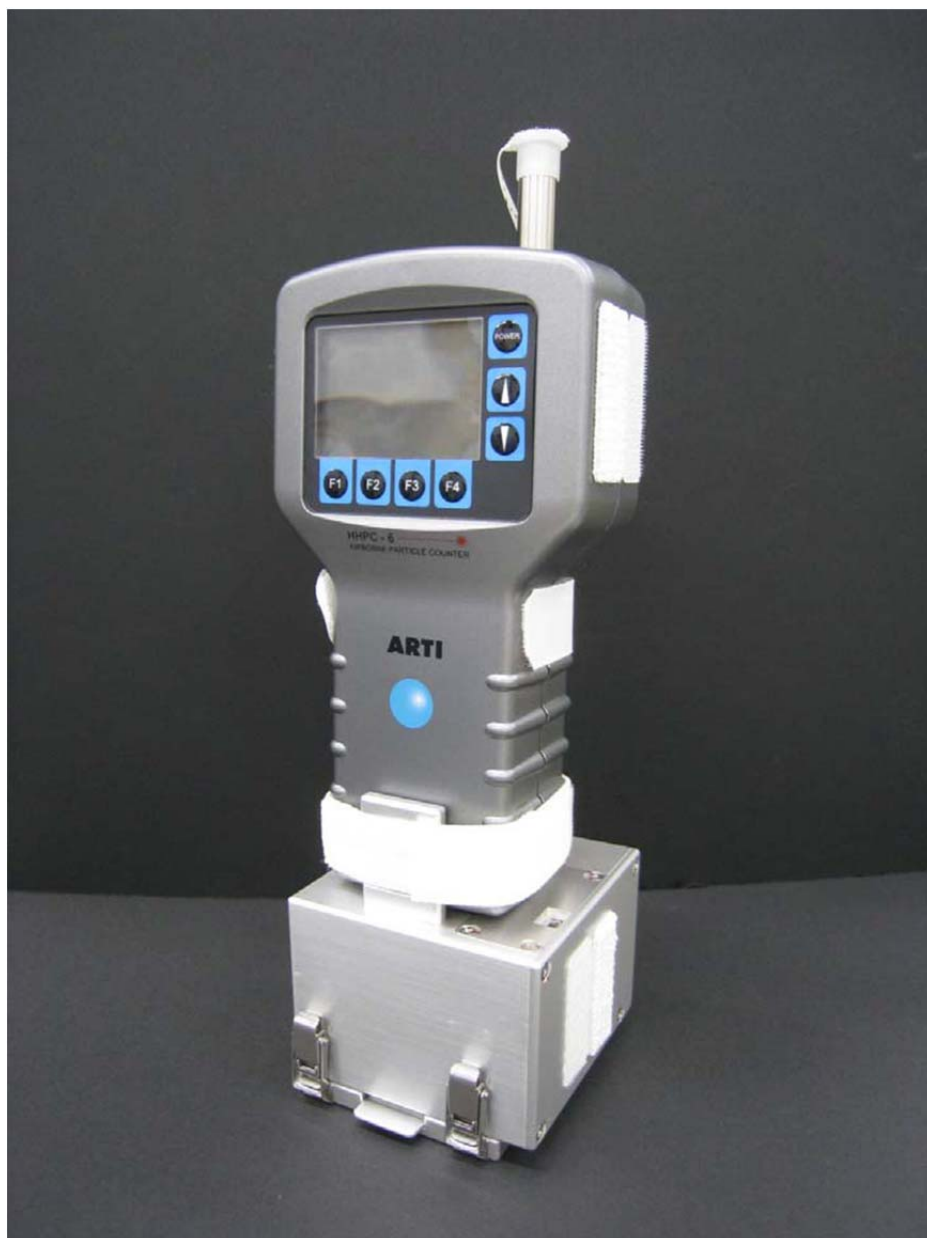
Fig. 2.7-1 Particle Counter (Silver part at the bottom is the size D battery box.)
