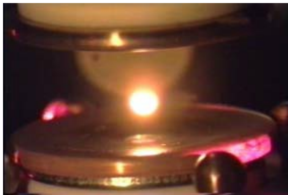
Fig. 3.5-1 Floating and heating in Electrostatic Levitation Furnace on earth
