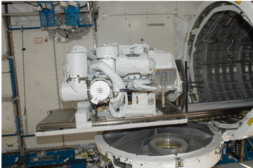
Fig 2.3.2-1 KIBO Airlock January 6, 2010 (SAF is attached on the slide table. Photo from overhead side)
