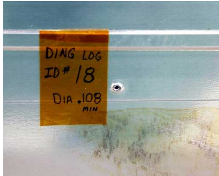
Fig 2.1.6-1 The space debris impact on the Space Shuttle Atlantis's right payload bay door (2.5mm in diameter)
