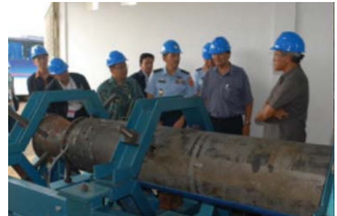
Body Tube Rocket-RX.420 LAPAN, Steel S45C
