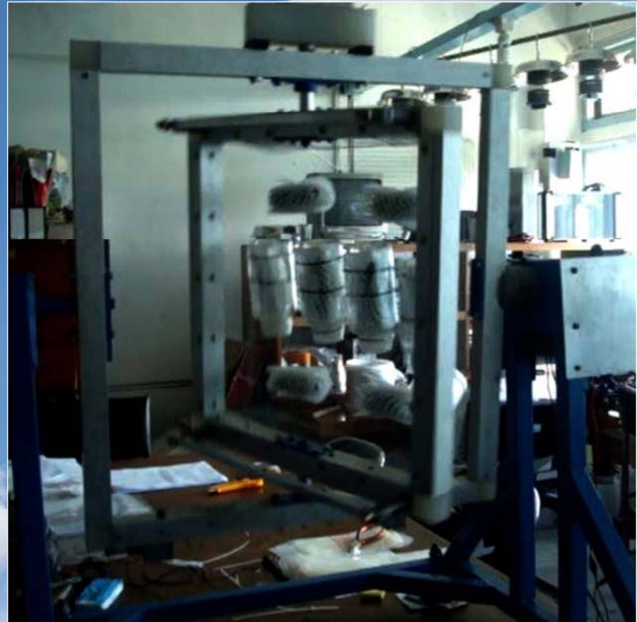
3D clinostat developed at ITB
