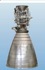
LE-6B LON-HS Engine Thrust: 14.0 tons (vacuum) for H-I/A and H-II/B Launch Vehicle Second Stage
