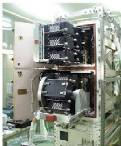
International Space Station (ISS) Cell Biology Experiment Facility (CBEF) aboard "Kibo" Module
