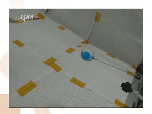
In this image, after injecting water in the oil, water (blue) remains inside the ball of silicon oil (colorless).
