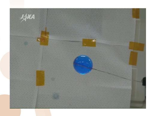
In this image, upon injecting oil in the water, although unclear on initial observations, the silicon oil (colorless) stays inside the ball of water (blue).
