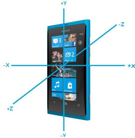
Figure 2.5. The acceleration data collected in 3 direction (along 3 axis)
