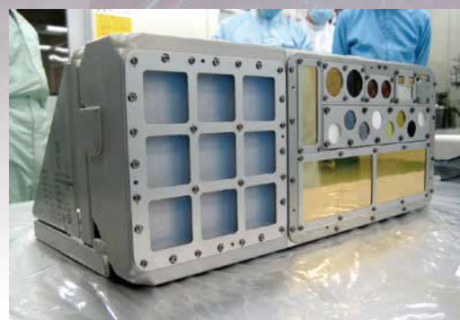
Micro-Particle Capture Experiment (MPAC) Device and Space Environment Exposure Device (SEED) attached to the Space Environment Data Acquisition Equipment-Attached Payload (SEDA-AP) of "Kibo"
