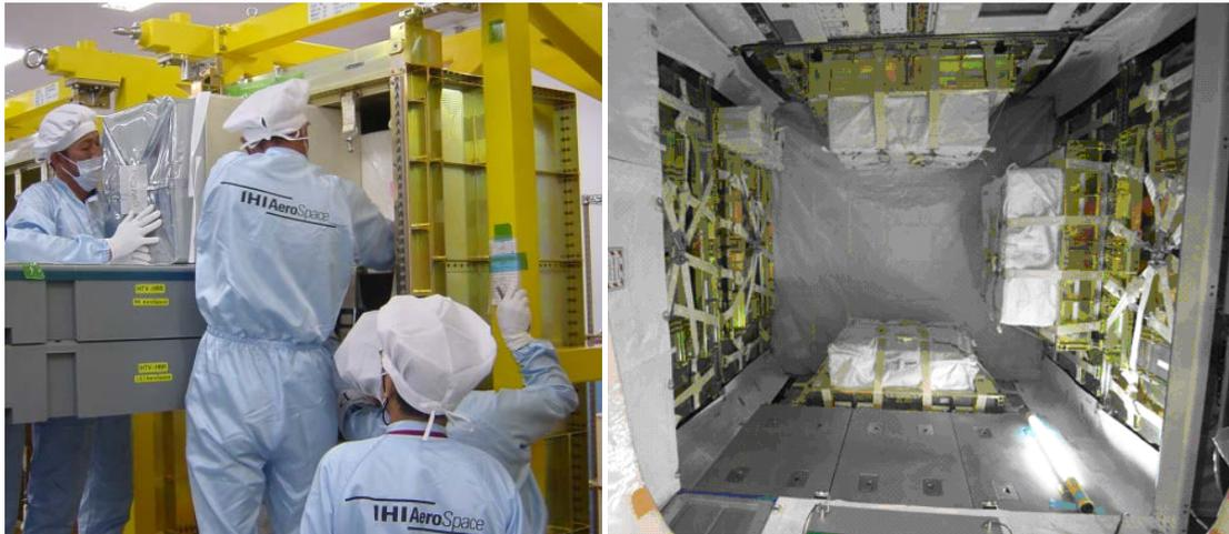
Figure 4.1-3 CTBs being installed in an HRR
