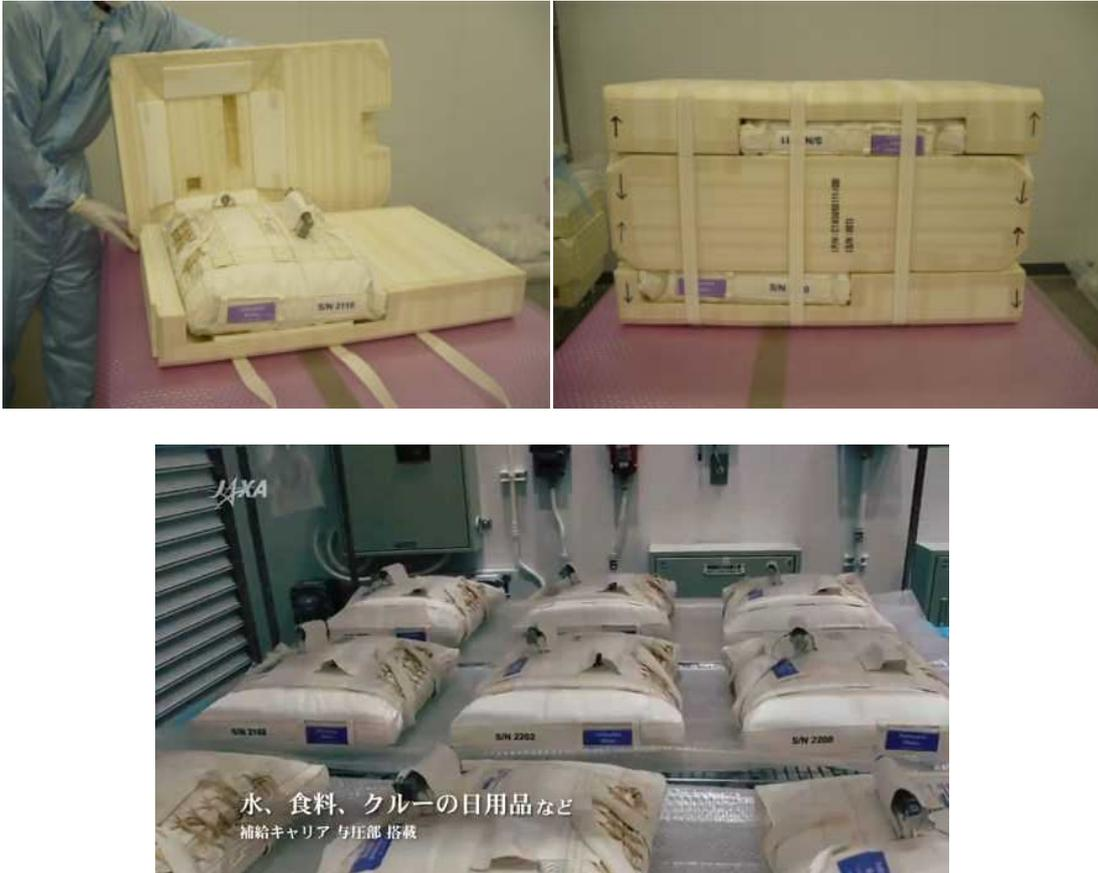
Figure A2-2 Above: A water bag (CWC-I, labeled purple) (left) and the packed image (right) (In the HTV2 mission)
