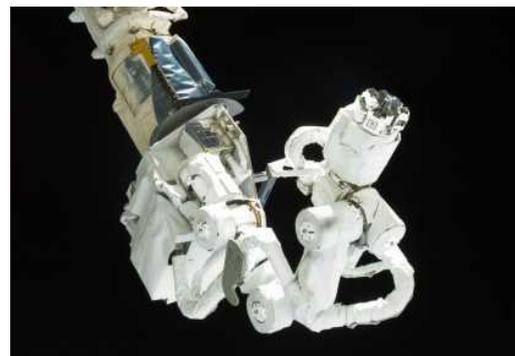
Figure A2-10 Small Fine Arm (SFA) of the Kibo's Remote Manipulator System (JEMRMS) (Delivered by the HTV1)
