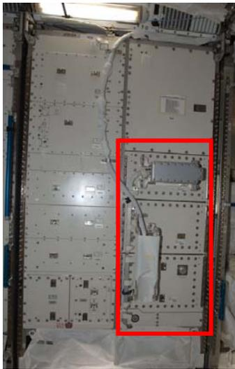
PROX communication systems are installed on the right side of the ICS/PROX Rack, which is located on the zenith port side on the Kibo's PM.
