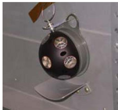
The Laser Rader Reflectors (LRRs) are located on the nadir side of the PM. The reflectors will reflect the lasers beamed from the HTV's Rendezvous Sensor (RVS) when the HTV approaches from the nadir side of the ISS.
