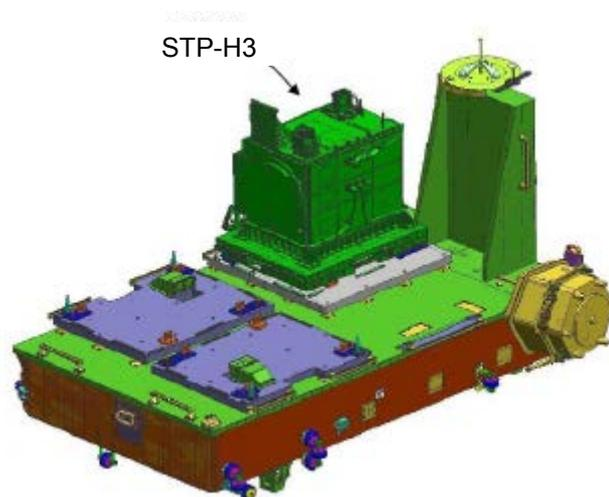
Figure 1.3-4 Waste cargo layout on the EP (image courtesy of NASA)
