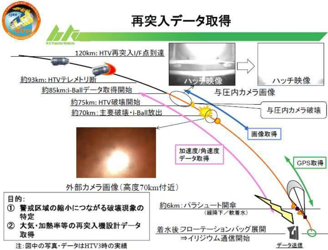
Figure A3-2 Planned data acquisition by the i-Ball during reentry
