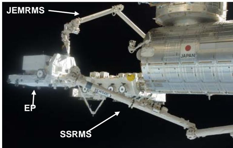
The EP being handed over from the SSRMS to the JEM Remote Manipulator System (JEMRMS) for temporary installation on the EF (image of HTV1)
