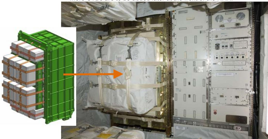
Figure 4.1-4 Left: CTBs installed at the front of a rack (HTV2)
