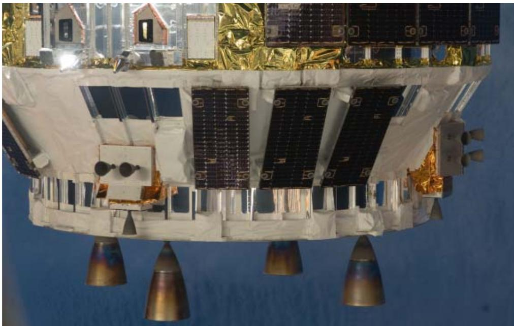
Figure A1.5-3 Propulsion Module Photographed from the ISS (HTV1)
