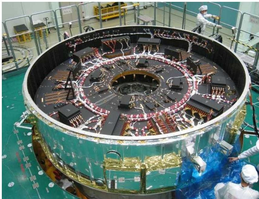
FigureA1.4-2 Avionics Module (Top View) (HTV2)
