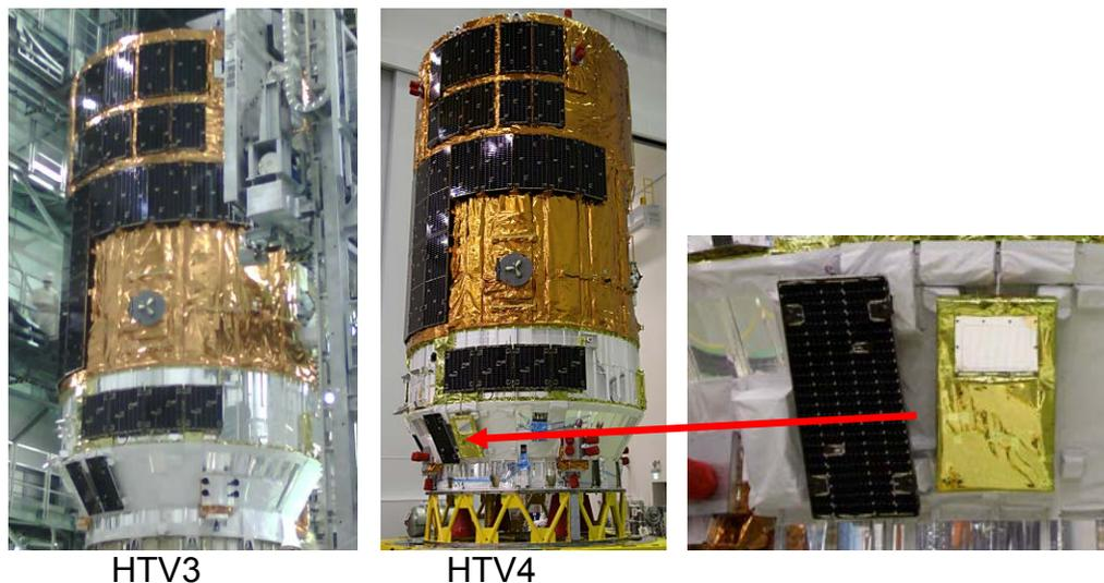
Figure 5.2-1 The surface potential sensor “ATOTIE-mini” (Advanced Technology On-orbit Test Instrument for space Environment - mini)
