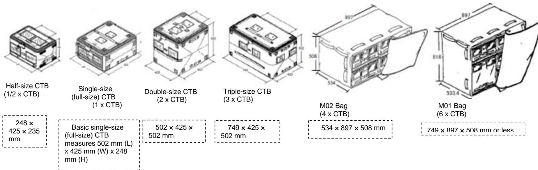
Figure A2-1 Several sizes of CTBs are available to transfer goods to the ISS
