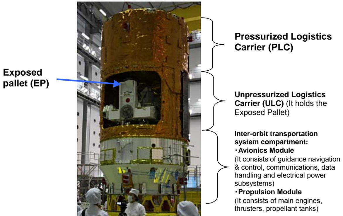
Figure 1.1-1 Configuration of “KOUNOTORI” (photo: HTV4)
