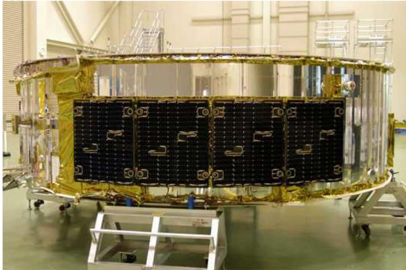
Figure A1.4-1 Avionics Module (Side View) (HTV1)
