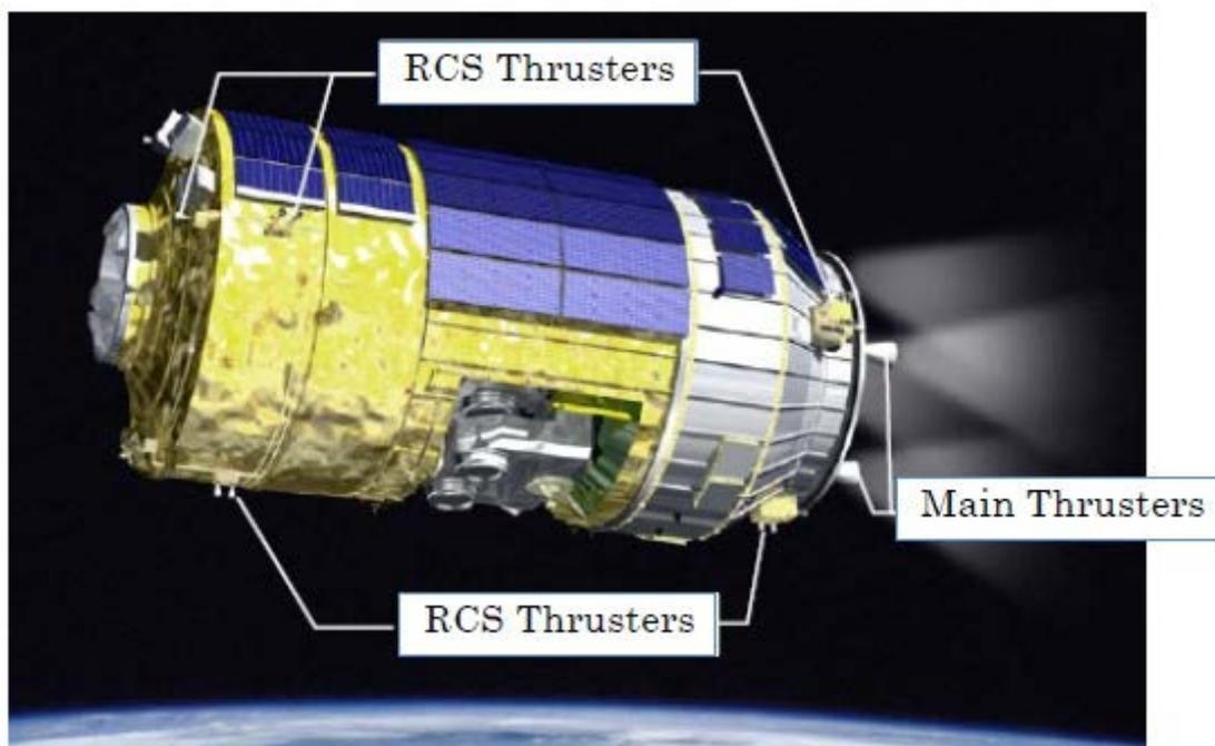
Figure A1.5-4 Locations of Main Engines and RCS Thrusters
