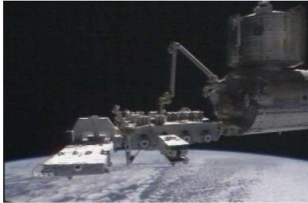
EP being temporarily installed to the edge of the EF (HTV1)
