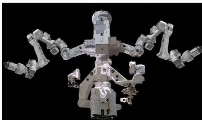
Figure 4.2.3-2 SPDM called "Dextre" (Credit: NASA/CSA)
