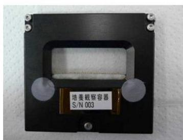
Chamber for Aniso Tubule experiment (plant seeds are set inside)
