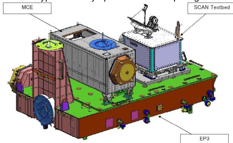
Figure A1.3-3 Exposed Pallet-Multi-Purpose (Type EP-MP)
