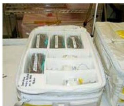
Food, daily commodities and experiment samples are packed in the CTBs and installed in the HRRs.
