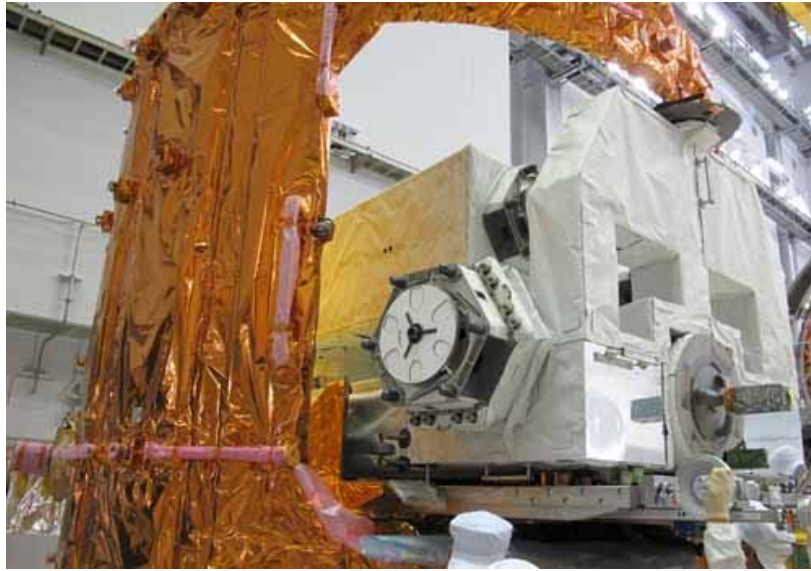
Fig. 1.3.5-2 Exposed Pallet being installed in the ULC
