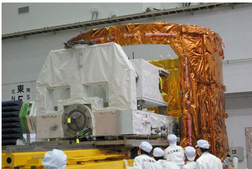
Fig. 1.3.1-2 Exposed Pallet being installed in the ULC
