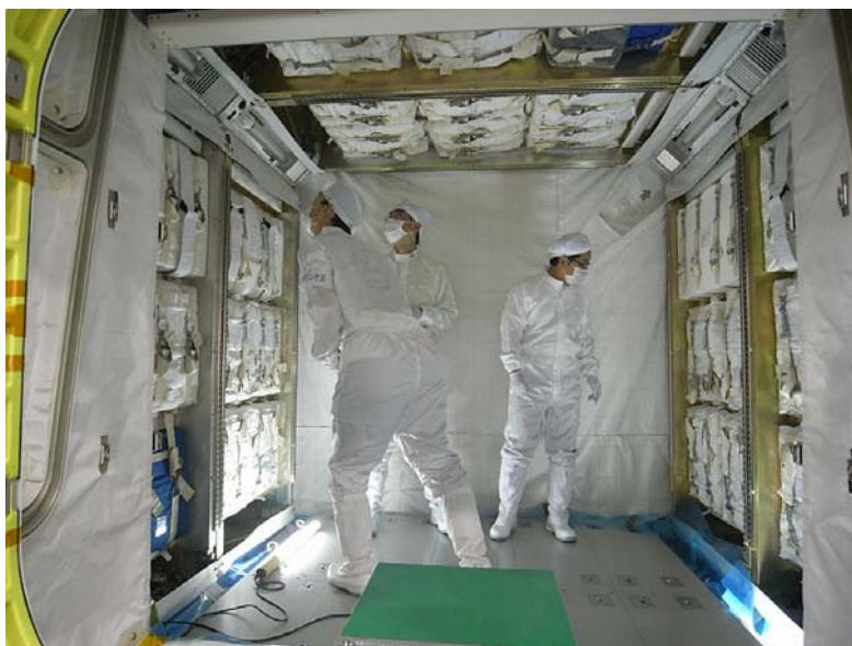
Fig. 1.3.5-1 Internal View of the PLC
