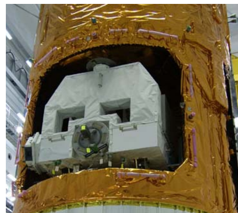
Figure 1.2.2-3 EP Installed into the ULC (HTV-1)
