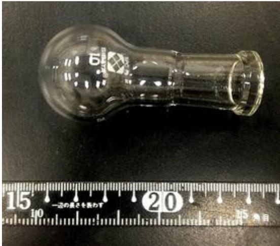
Fig. 1 A picture of round-bottomed glass flask
