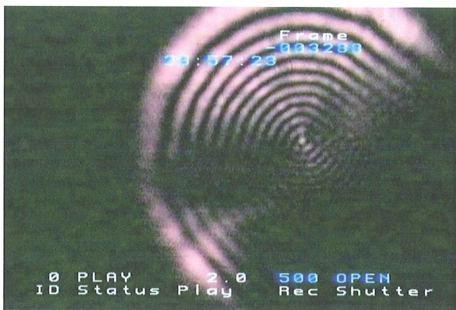
Fig.4 Interferometric Image of a droplet suspended by optical tweezers
