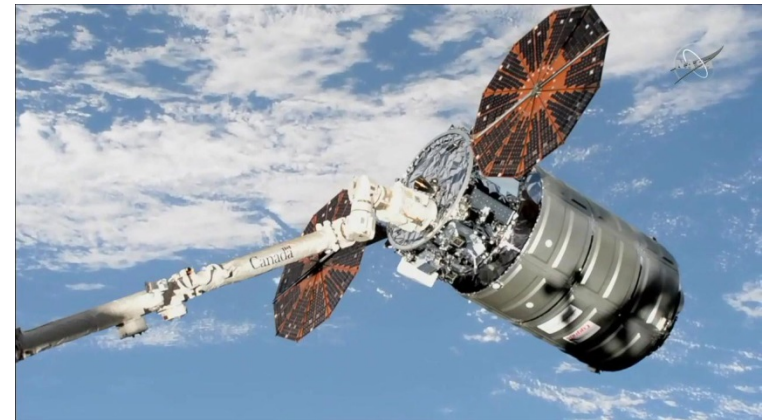
SRMSで把持されたNG-10(出典: JAXA/NASA) https://blogs.nasa.gov/spacestation/2018/11/19/u-s-space-freighter-captured-by-nasa-astronaut/
