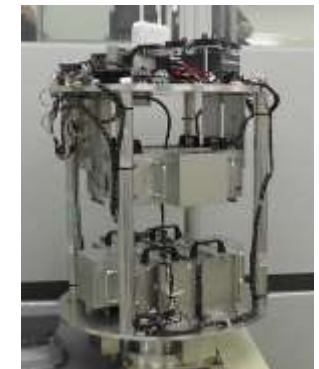
Short-arm centrifuge for mice (R=15cm)
