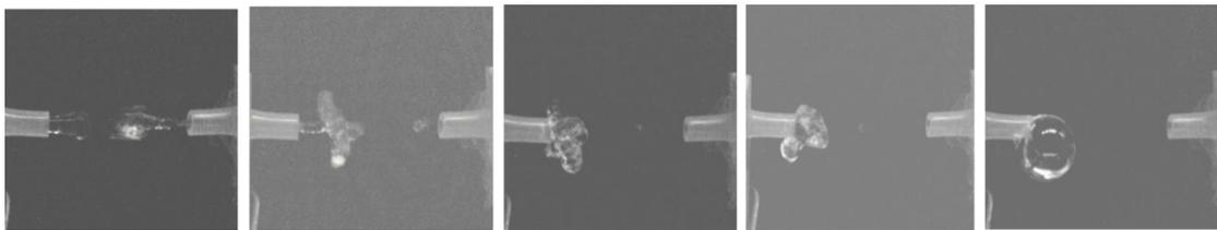
A next photo shows a droplet formation system. The spring is shortened with the weight of a clay lump under normal gravity. When gravity disappears, the spring extends and a droplet is pushed out from the nozzle by the extruded air with the power of spring.
