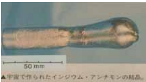
Figure 4. An InSb crystal grown by the floating zone method in space.
