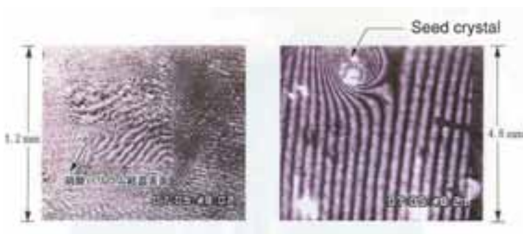
Figure 1. In-situ observation of the liquid density around a growing crystal by interferometry.
