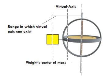
Gyroscope's center of mass
