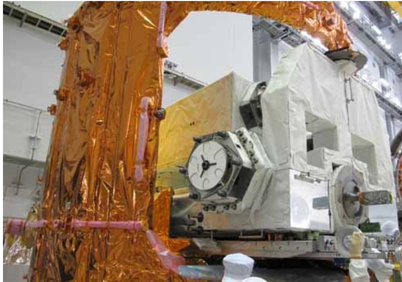
Fig. 1.3.5-2 Exposed Pallet being installed in the ULC
