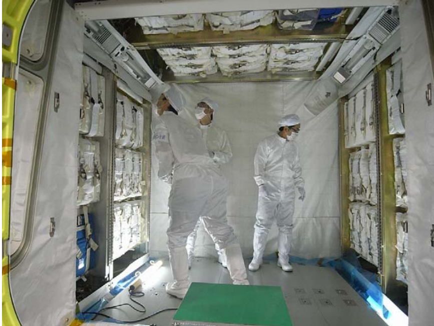
Fig. 2.3-1 PLC (Resupply racks with cargo transfer bags being installed inside the module)
