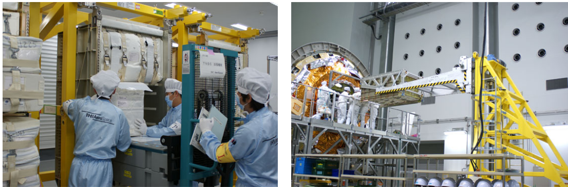
Fig. 1.3.1-1 Cargo Transfer Bags (CTBs) being installed in the HTV Resupply Racks (HRRs) and an HRR being loaded into the PLC (Launch Processing on the HTV-1 Mission)
