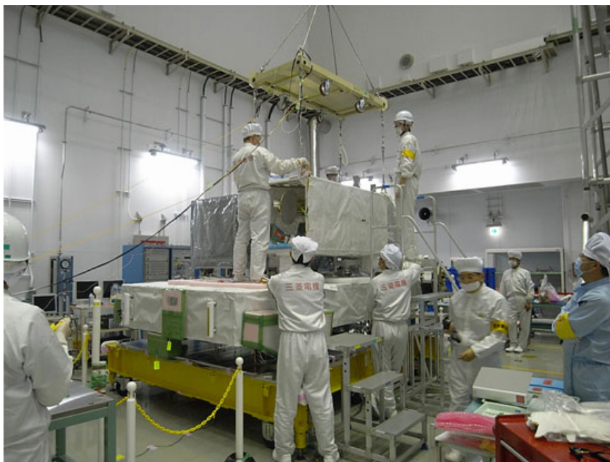
Fig. 2.3-2 EP (External payloads being installed on the pallet)
