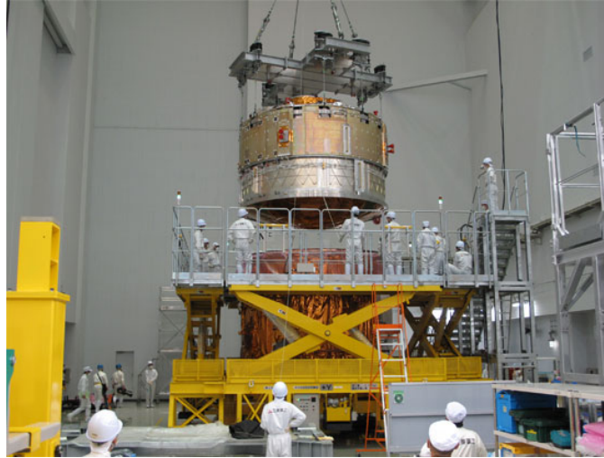
Fig. 1.3.1-3 PLC and ULC being mated
