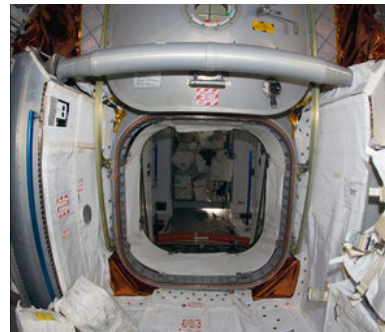
View of the vestibule between Harmony and the MPLM; The MPLM being docked to the CBM, located at the nadir side of Harmony
