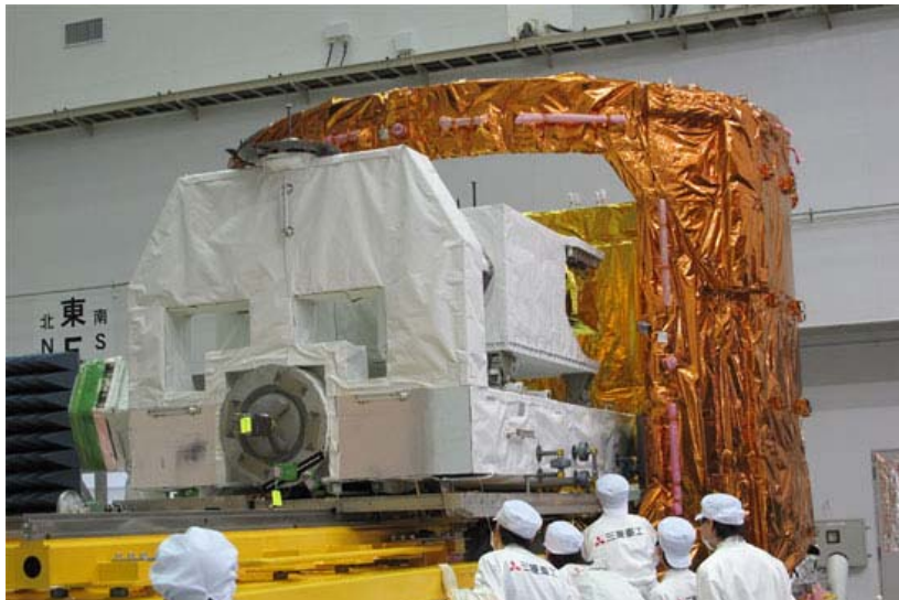
Fig. 1.3.1-2 Exposed Pallet being installed in the ULC
