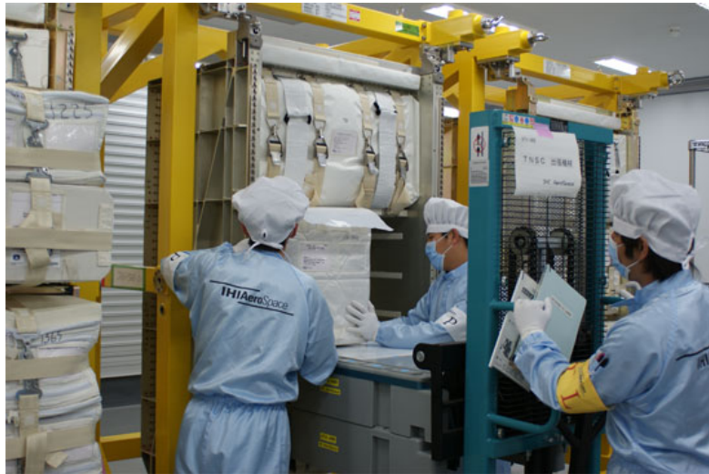
Fig. 2.3.1-4 CTBs being installed in HRRs
