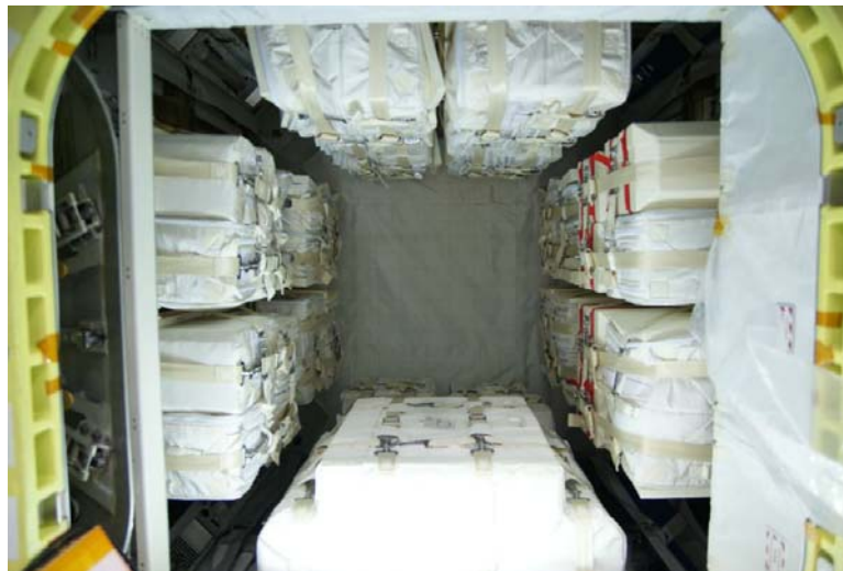
Fig. 2.3.1-6 Cargo Layout inside the PLC (HTV-1) (*CTBs are also installed on the front side of the HRRs)
