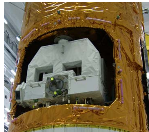
Figure 1.2.2-3 EP Installed into the ULC (HTV-1)
