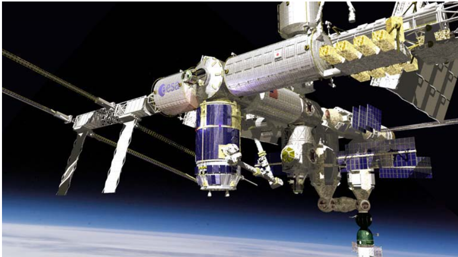
Fig. 1.3.4-4 SSRMS Moving the HTV to the Berthing Position
